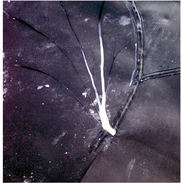
Figure 7. Cracking of the geomembrane.
