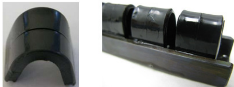
Figure 5. Example of a Bent strip samples prepared for ASTM D1693 immersion testing
