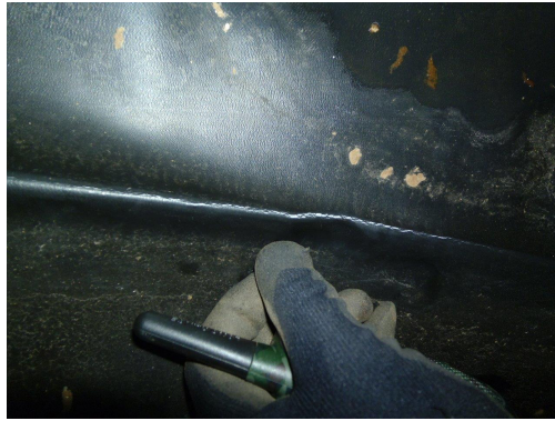
Figure 1. Damage at the top of a fold in the liner
