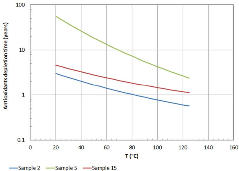
**Figure 8** Antioxidant depletion using Arrhenius model, from exposure to chlorine water
