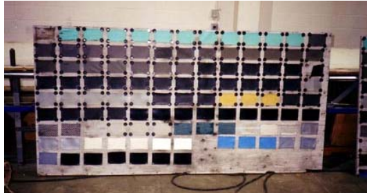
Figure 1 One of three natural weathering sample racks after 6 years of exposure.
